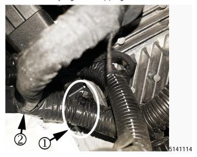
3. Remove the harness clip from the (1) from the bracket to allow access to the harness junction (2).
