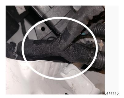
4. Apply anti-abrasion tape to the junction as shown, being sure to cover the harness completely, especially at the center of the junction where there is no convoluted conduit. The anti-abrasion tape should extend approximately 1 inch (25.7mm) out to each branch of the harness.
