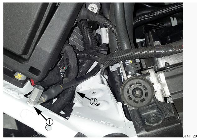
2. Remove the battery negative stud (1) to gain access to the harness junction (2).
