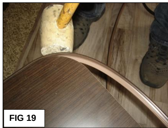
FIG 18: Make sure the edge trim is flush to the table edge. Gaps like that shown here need to be pounded flush using the rubber mallet.
