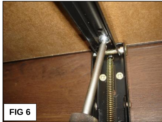
FIG 5: Remove the black screw at the front of each long table bracket.
