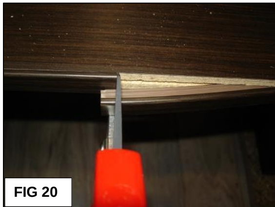
FIG 20: When you get around the rear of the table, use trim shears to cut the molding.
