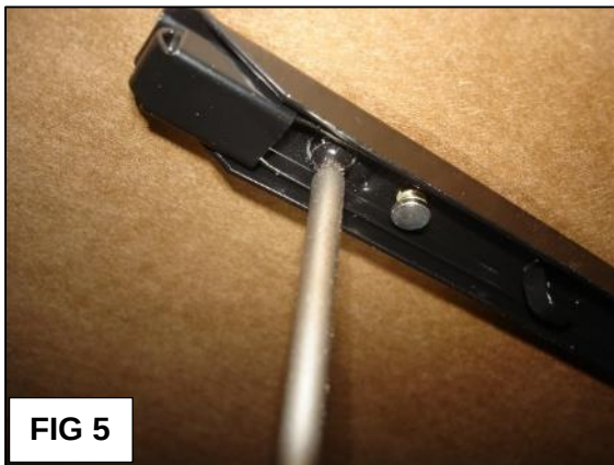
FIG 5: Remove the black screw at the front of each long table bracket.
