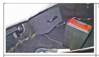
7. Remove the backing paper from the bottom and press the two prepared foam blocks onto the inner two ISOFIX anchor brackets.
