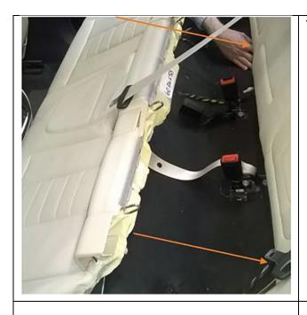
11. Reinstall the rear seat bench according to the repair instructions REP-TAT-P-5226-02-G01 "Installing the rear seat bench".
