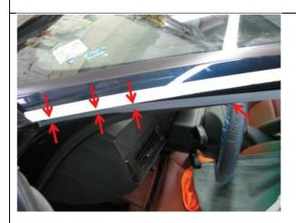
5. Apply Teflon tape to the preheated area as shown.
