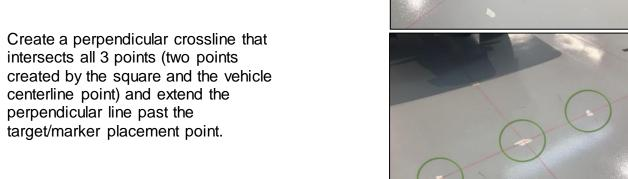
6. Refer to the **Blind Spot Monitor** Calculator or the applicable Repair Manual for this measurement. On the perpendicular crossline, mark the distance from the vehicle centerline where the target will be placed.
