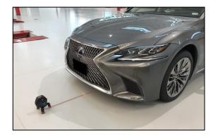
Place the laser target from the SST kit (PN 00816-00103) on the REAR vehicle centerline mark.
