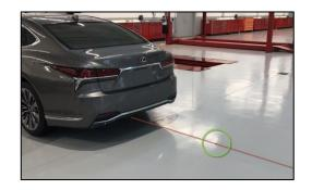
Hint: The example photo is displaying the perpendicular crossline point in the **rear** of the vehicle for Blind Spot Monitor, but this tip can also be used for Forward Recognition Camera, where this point will be at the **front** of the vehicle.
