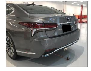
5. Align the laser with both vehicle centerline marks.
