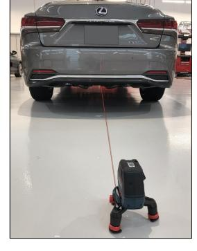
6. Create the perpendicular line using the 90-degree laser.
