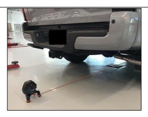
Place the laser target from the SST kit (PN 00816-00103) on the FRONT vehicle centerline mark.
