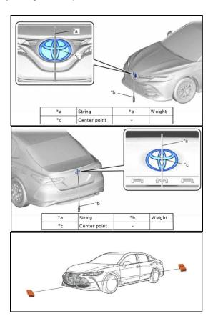
Creating a Perpendicular Crossline - Marking a perpendicular line off the vehicle centerline is the
