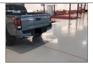
B. Creating a Centerline Using a 90-Degree Laser (for Forward Recognition Camera and Front Millimeter Wave Radar)
