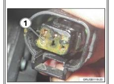
2. Remove the connector and check the pins in the connector for traces of water or corrosion.
