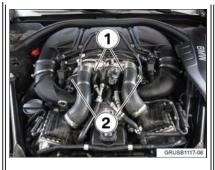
Insert the borescope to the inside (1) and outside (2) of the induction pipes.
