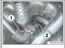
Insert the borescope downward towards the turbocharger oil return pipes.
