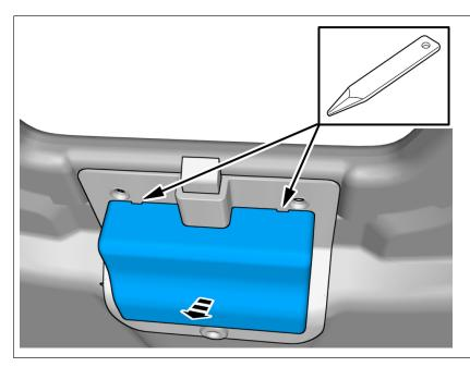
**Use:** Interior trim remover Remove the part carefully Remove the marked part.
