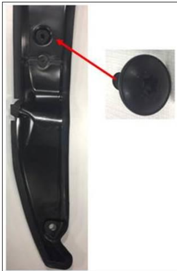
Figure 3: Installation of hexagon socket head panel bolt to the new fender end plate.
