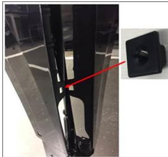
Figure 2: Installation of the expanding nut into the fender.
