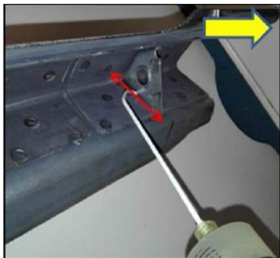
Figure 7a: Cut-away illustration of the internal area for the Krytox™ application on front bracket.
