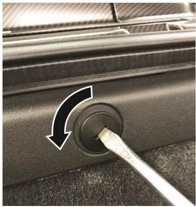
Installing these fasteners is really easy; just press them into the threaded studs.
