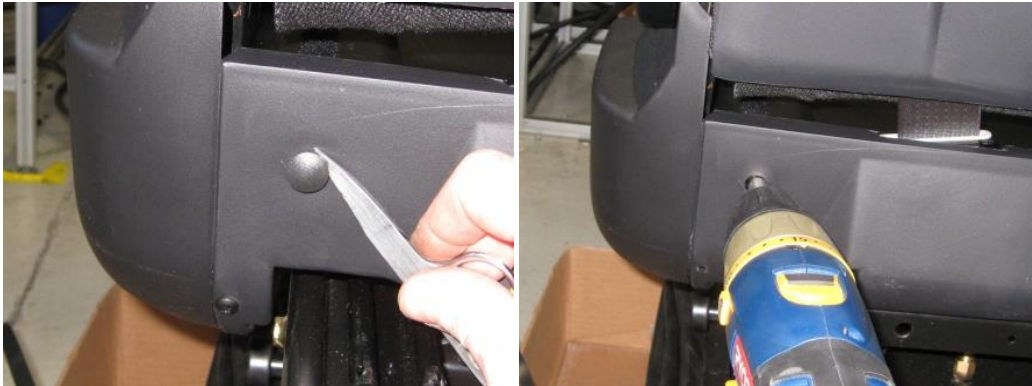
Figure 3: Rear trim panel, remove hole plugs (left), remove trim panel (right)
