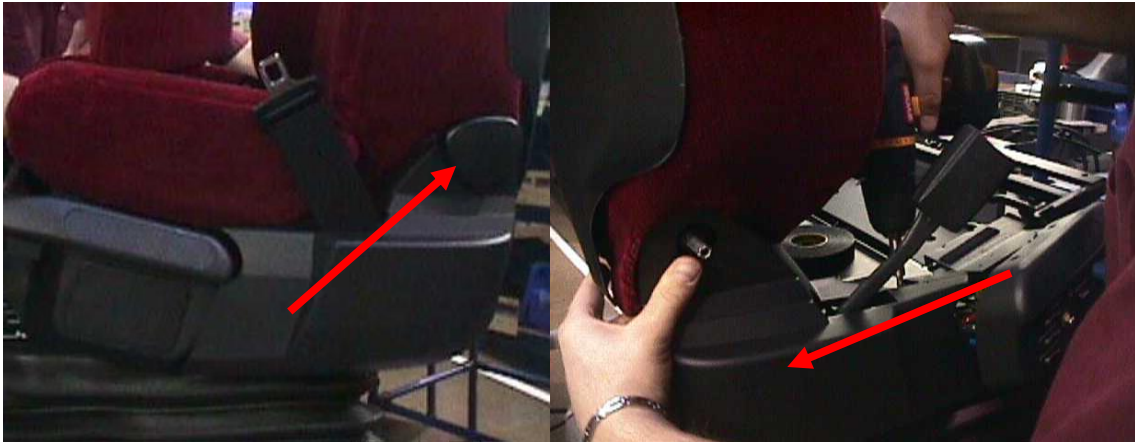
Figure 4: Seat belt buckle bolt access, hand wheel (left), rear side trim (right)
