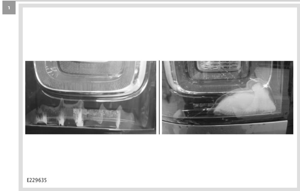
Staining, tarnishing, and/or contamination on the outer lens.
