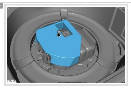
Install the protective foam block to the air suspension compressor assembly.
