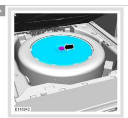
Remove the spare wheel retainer and cover.
