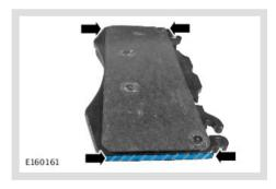
Apply long life lubricating grease to both ends of the brake pads.
