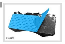
Gently remove the brake pad backing.
