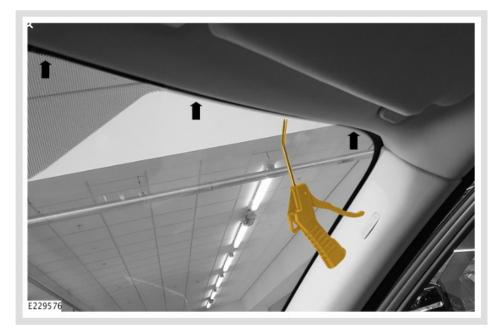
Use an air blower to blow compressed air around the edge of the inner side of the windshield as shown.
