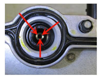
If you find the above PCV orifice is plugged or restricted use a 1.8mm drill bit (hand use only) to clear the orifice.
