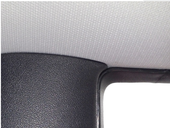
✓ Figure 2 (Fit is tight, no gap)
