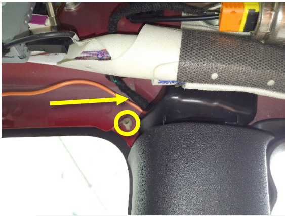
✓ Figure 4 (Harness forward of the clip)
