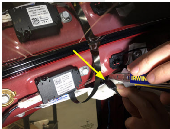
Figure 6 (Carefully cut the tape)
