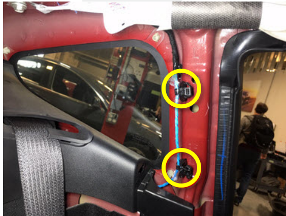
Figure 8 (Cut clips, not electrical harness)
