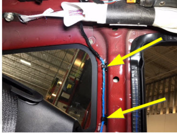
Figure 7 (C-Pillar cable tie clips)
