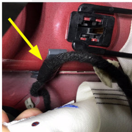
Figure 10 (Secure clip to harness)
