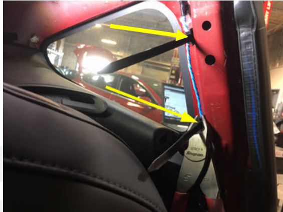
Figure 9 (Secure the harness in position)
