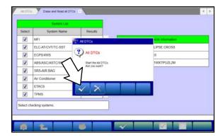
c. A window will pop up asking you to confirm DTC erasing. Click the check mark in the dialog box for DTC erasing and reading to begin.
