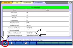
d. If the Software Part Number listed is **not** at the latest level (shown in the **"ECU Reprogramming Chart"** in this TSB), proceed with the next step. Click the Home button to return to the System Select screen.
