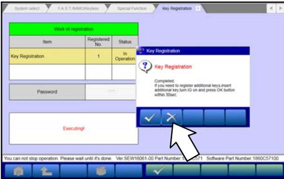
d. The Key Registration dialog box will show a "Completed" message when a key is successfully registered. Repeat the procedure shown in the message until all keys are registered.
