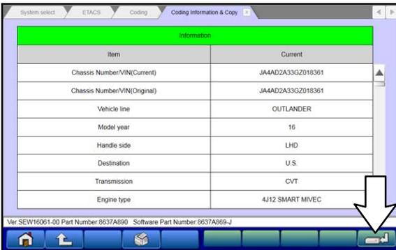
d. Click the Save button to save the ETACS coding data ".kon" file from the old ETACS to the MUT-III HDD.
