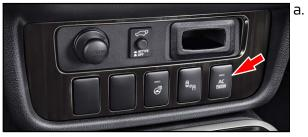
. To enable power to the 120V AC outlets on the Outlander PHEV, press the "AC 1500W" switch in the center console.
