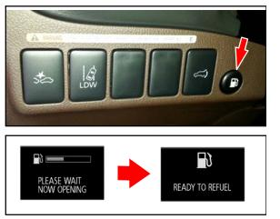
• Push the fuel door release button on the lower dash left of the steering wheel.
