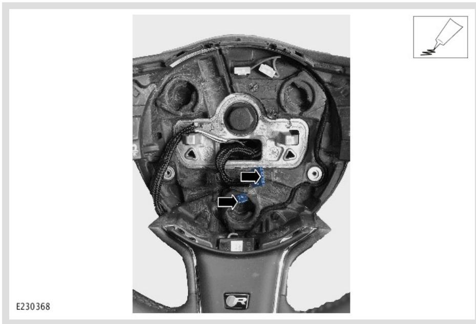
Apply the Nyogel to the front of the steering wheel control switch electrical connectors.
