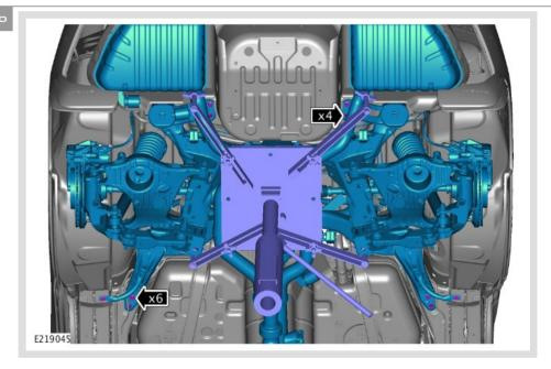
Tighten the subframe support plate retaining bolts (6) and nuts (4).
