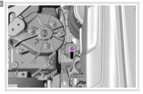
Loosen the right engine mount nut.
