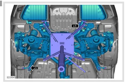
Loosen (only) the subframe support plate retaining bolts (6) and nuts (4).
