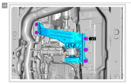
Tighten the 5 transmission mount fasteners.
