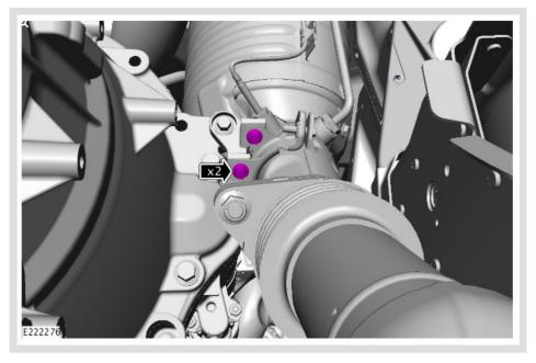
Loosen the 2 Diesel Particulate Filter (DPF) fasteners.
