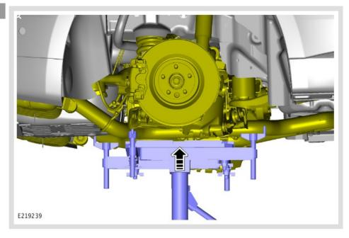
Use the transmission jack to raise the subframe into the correct position.
