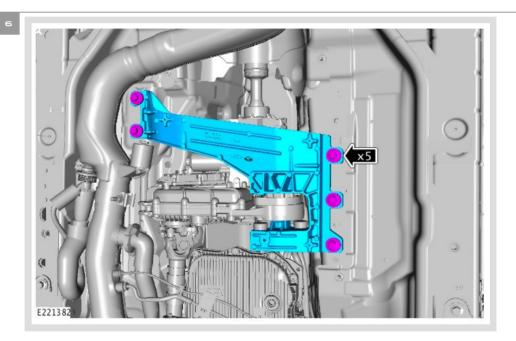
Loosen the 5 transmission mount fasteners.
