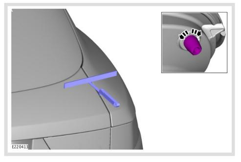
Use a suitable straight edge and a feeler gauge to set the tailgate alignment to 2.5 mm under flush.
