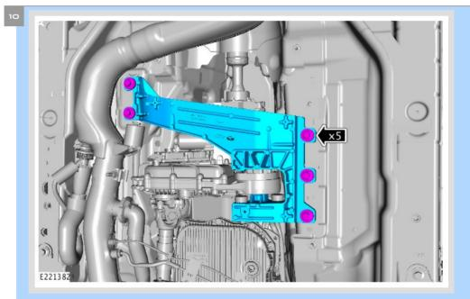
Tighten the 5 transfer case support bracket fixings.
