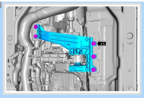
Loosen the 5 transfer case support bracket fixings.
