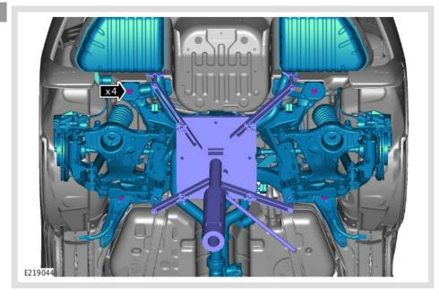
Tighten the subframe retaining bolts.
