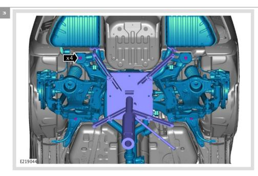
Support the rear subframe assembly with a suitable transmission jack.
