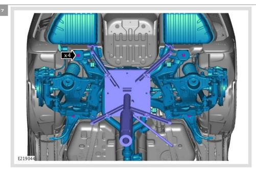
Install the 4 new subframe retaining bolts but do not tighten fully at this time.
