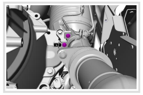
Tighten the 2 DPF fasteners.
