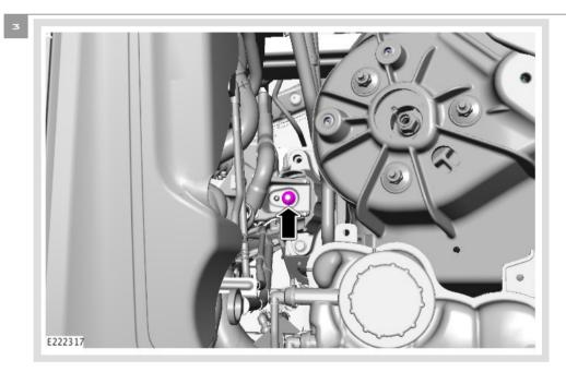
Loosen the left engine mount nut.
