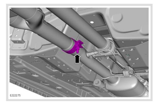
Tighten the exhaust clamp.
