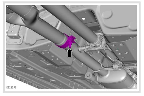
Loosen the exhaust clamp.
