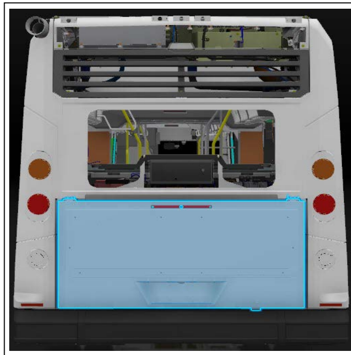
Figure 1 - Rear Engine Access Door
