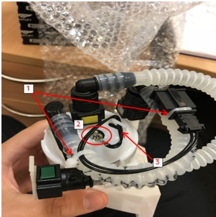
Figure 2 - Old fuel filter harness (Version 1)
