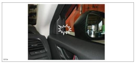
The rattle noise may be caused by insufficient holding force of the glass run channel. To increase the holding force, the shape of glass run channel has been changed and non-woven pads have been attached to the glass run channel.
