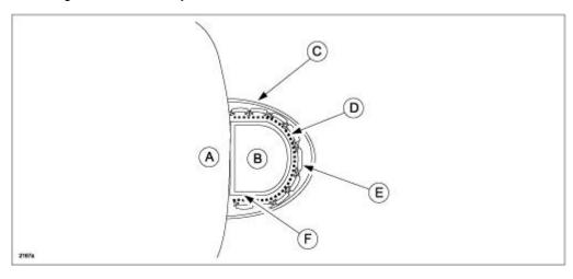
NOTE: Ensure the aluminum foil tape (F) is inserted into the edges of the molding (B) as shown below.
