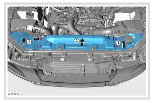
Remove the engine compartment front trim covers.
