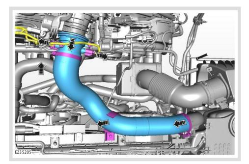
Remove and discard the charge air cooler hose.
