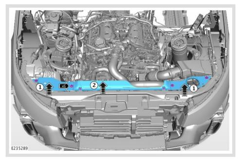
Remove the engine compartment front trim covers.
