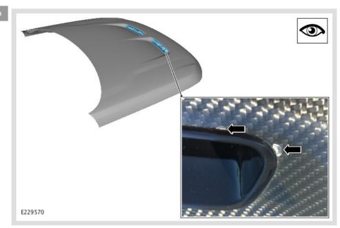
Inspect the hood for delamination in the area surrounding the hood vents.
