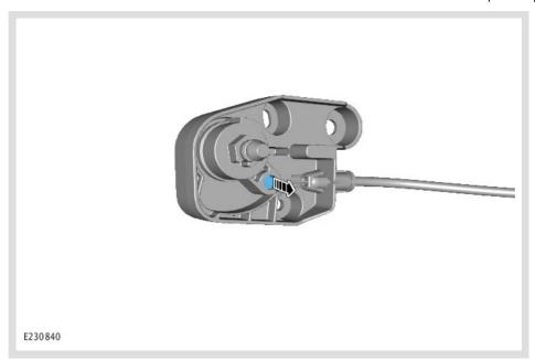
Release the hood release cable from the hood release mechanism.
