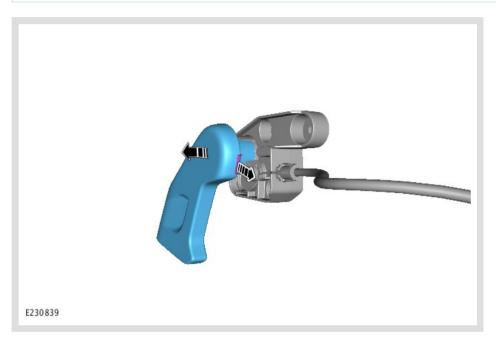
Remove hood interior release lever from the hood release mechanism.
