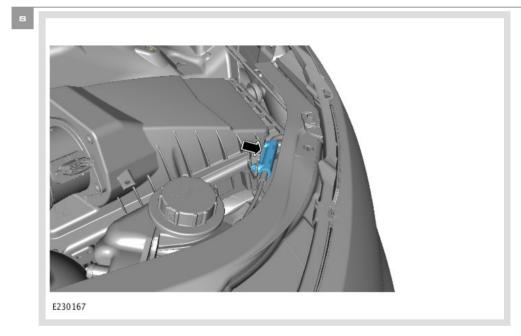
Release the hood release cable from the retainer.
