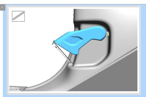
Open the hood and use a steel rule or similar engineer's scale to record the distance the interior release lever travels to operate the hood latches.
