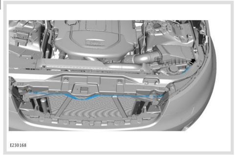
Remove the hood release cable from the vehicle.
