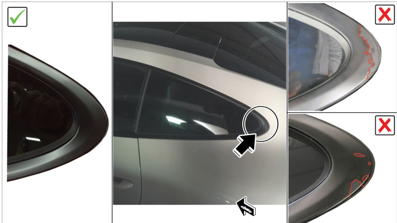
Checking and assessing moulding
