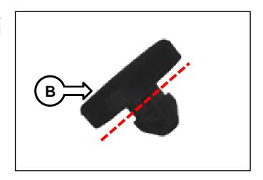
5. Install the new brake pedal stopper pad (D).
