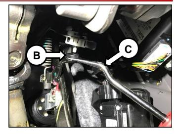
4. Cut the nub off of the removed brake pedal stopper pad (B) as shown and discard both pieces of the pad (B).
