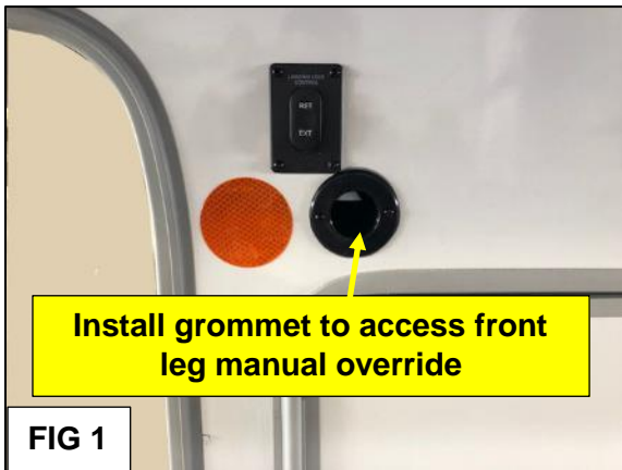
FIG 1: Grommet to be installed just above the forward compartment on the Off Door Side.
