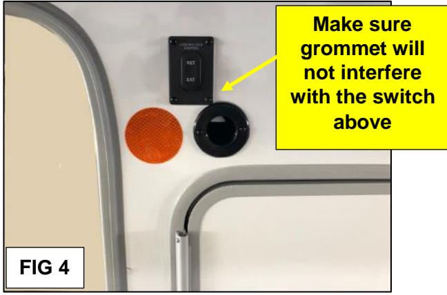
FIG 3: Measure back to the rear of the fifth wheel, from the front edge trim, 6-1/2 inches. Make another mark with the erasable marker, pen or pencil. This locates the center of the access hole for the manual override. FIG 4: Before drilling; make sure there will be enough clearance so the grommet does not come into contact with the switch or the compartment edging and that it sits flush to the outer wall.
