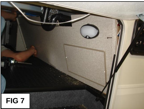
FIG 7: Pull the partition down to gain access behind it.
