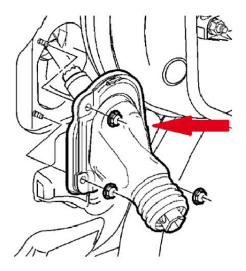
If no obvious issues are identified, remove the steering seal and inspect for any deformation, relpace as needed.
