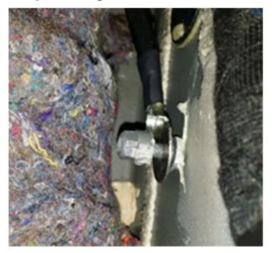
Category 3: P1AEE and P1AEF caused by a loose or intermittent orange high voltage cable connection
