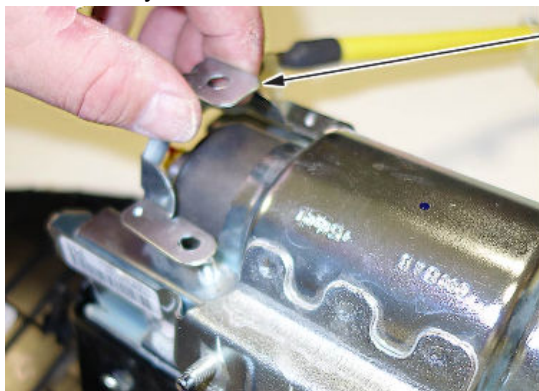
INFLATOR BRACKET Do not reuse.
