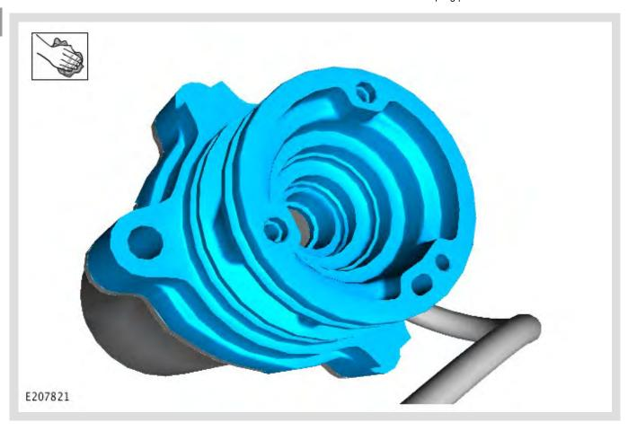
Use compressed air to make sure that the breather is clean and free from foreign material.
