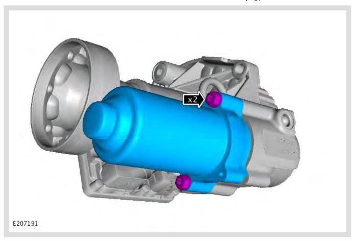
Remove the motor from the Active On-Demand Coupling.
