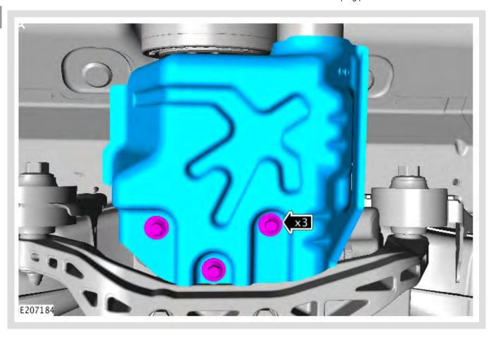
Remove the Rear Drive Unit (RDU) heat shield.
