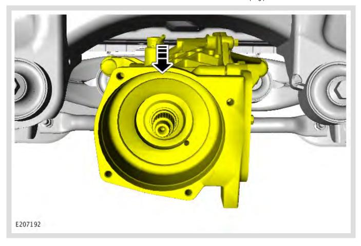
Lower the RDU to make sure all the RDU fluid is drained from the RDU.
