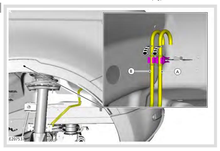
Disconnect the breathers from the retaining clips and position to one side.
