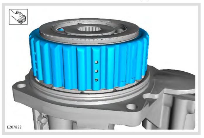
Clean the Active On-Demand Coupling using lint-free cloths and compressed air.
