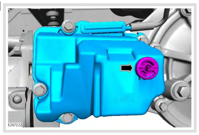
Install the Active On-Demand Coupling sump fill plug.
