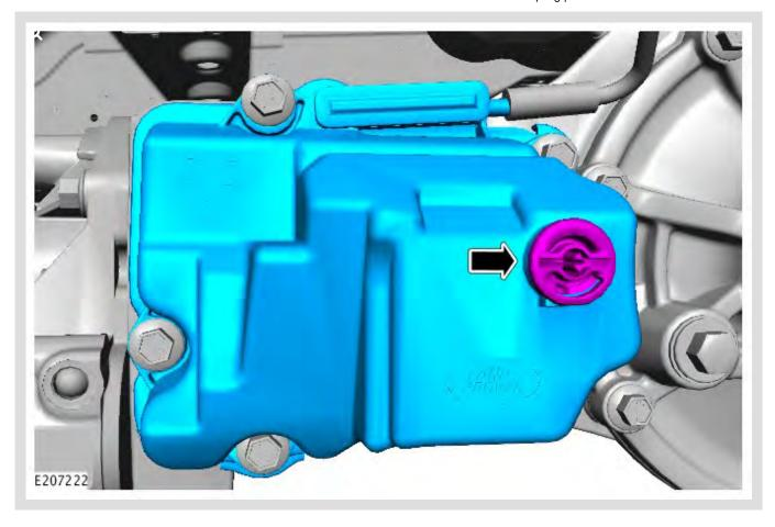
Remove the Active On-Demand Coupling sump fill plug.
