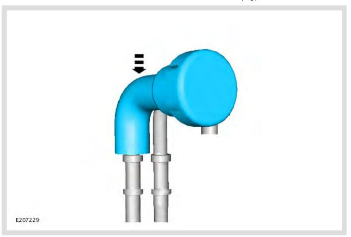
Install the new breather canister as shown.
