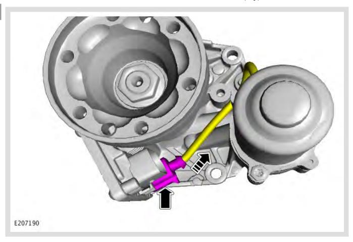
Disconnect the electrical connector from the Active On-Demand Coupling.
