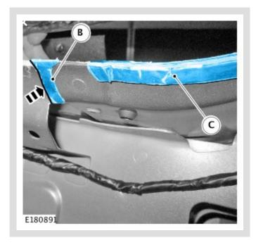
Locate and Install the seal pad against the panel edge shown.
