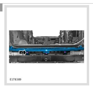
Remove the rear bumper cover center support bracket.
