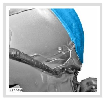
Note the correct position of the tailgate weatherstrip after being installed to the vehicle.
