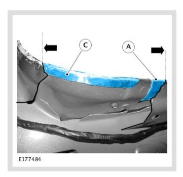
Install the seal pad on the vehicle in the area shown, locating the seal pad against the panel edges shown.
