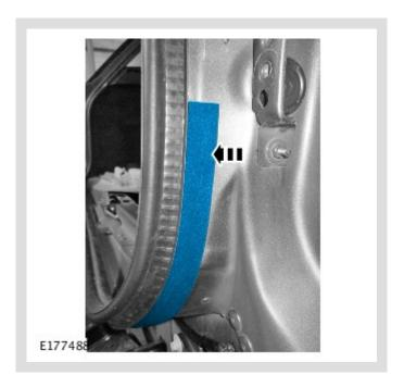
Make sure the foam strip is flush with the tailgate weatherstrip.
