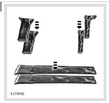
Stick two equal pieces together to make each piece twice the thickness.
