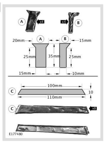
Use a suitable tool to cut the seal pad to the sizes shown.
