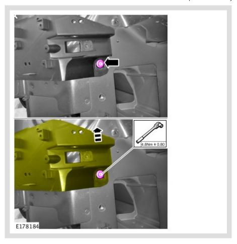
Install the rear bumper cover corner bracket holding at its uppermost position.
