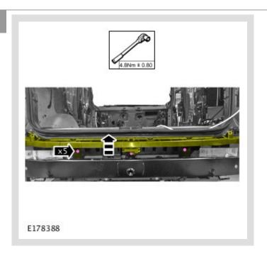
Install the rear bumper cover center support bracket holding at its uppermost position.
