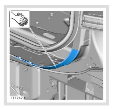
Use a suitable cleaning solution to clean the excess sealant from the vehicle in the area shown.
