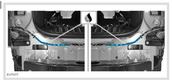
Use a suitable tape to wrap the rear electrical harness.
