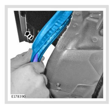
Use a suitable tool to spread the gap on the tailgate weatherstrip.
