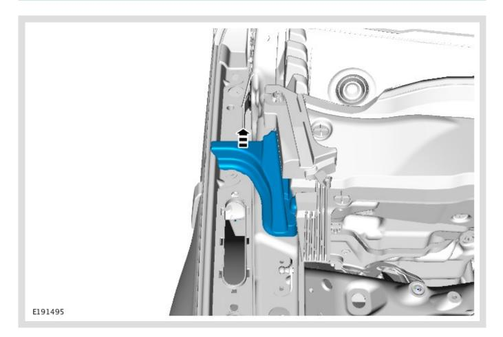
Remove and discard the under hood lower right-hand Noise Vibration Harshness (NVH) pad.
