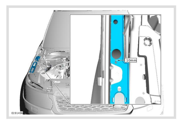
Drill a new 6.5 mm diameter hole as shown.
