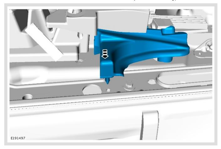
Install the new under hood lower NVH pad.
