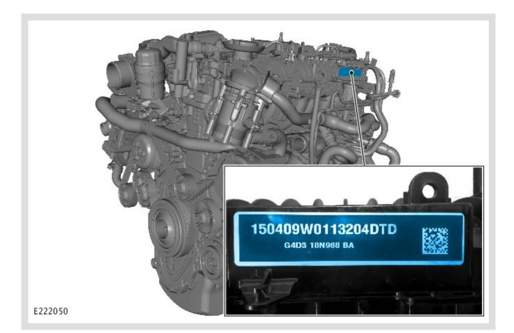
Locate and record the engine serial number.
