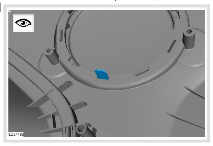
Inspect the mid-range speaker grille for the presence of a weld tower.
