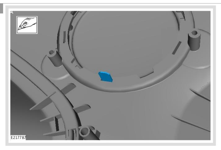
Use a suitable tool to remove the highlighted weld tower.
