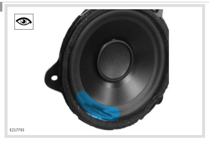
Possible damage to the mid-range speaker due to a weld tower present on the mid-range speaker grille.
