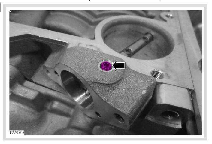
Remove the bypass valve set screw.
