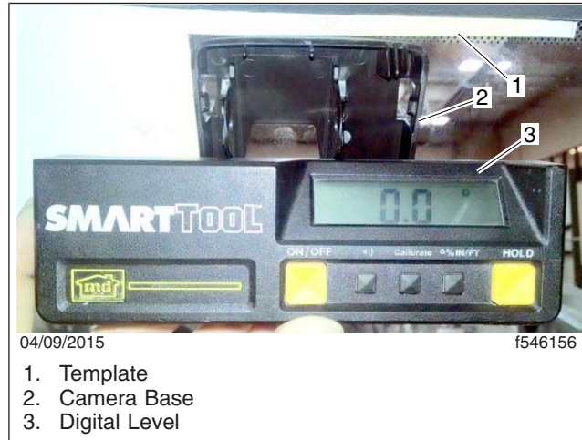
Fig. 11, Aligning the Base with a Digital Level
