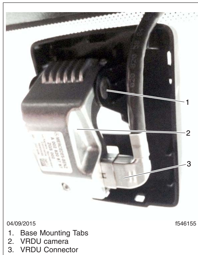
Fig. 13, VRDU camera Installed
