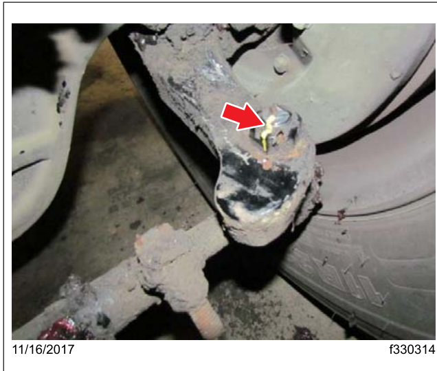
Fig. 3, Paint Mark to Identify Nut Rotation
