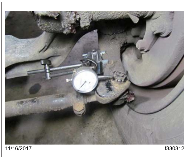
Fig. 1, Dial Indicator Mounting Position
