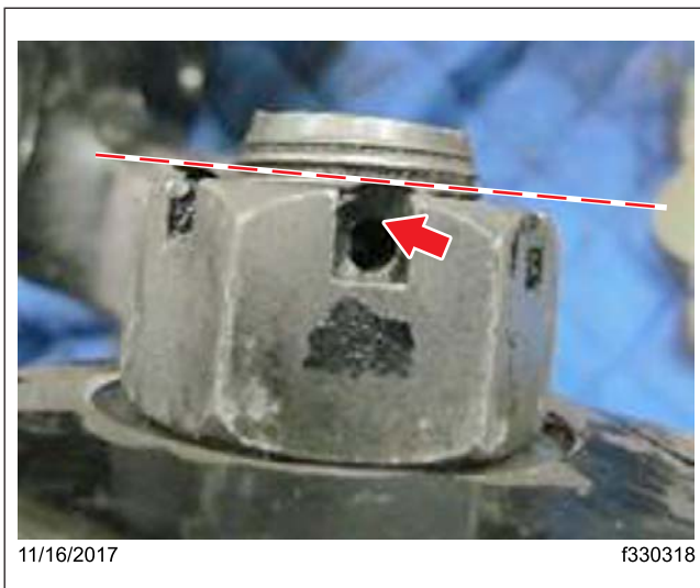
Fig. 7, Good Cotter Pin Hole Position
