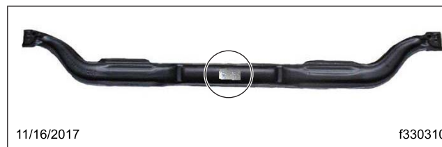
Fig. 9, Front Axle Identification Tag Location
