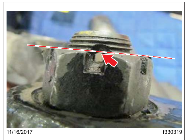
Fig. 8, Cotter Pin Hole at Maximum Height
