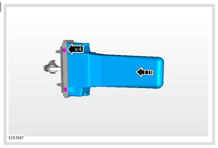
Install the new door check arm cover to the new front door check arm as shown.
