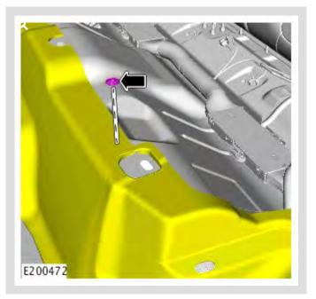
Remove the carpet retaining washer.
