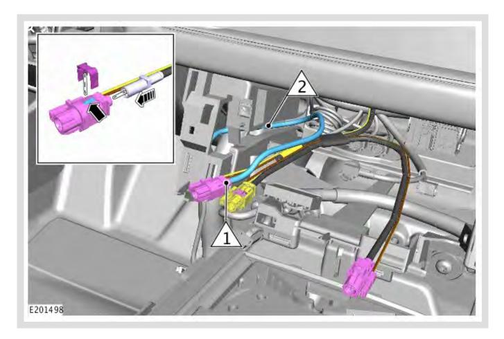
Install the new IMC rear link lead cable into the original electrical connector (1).
