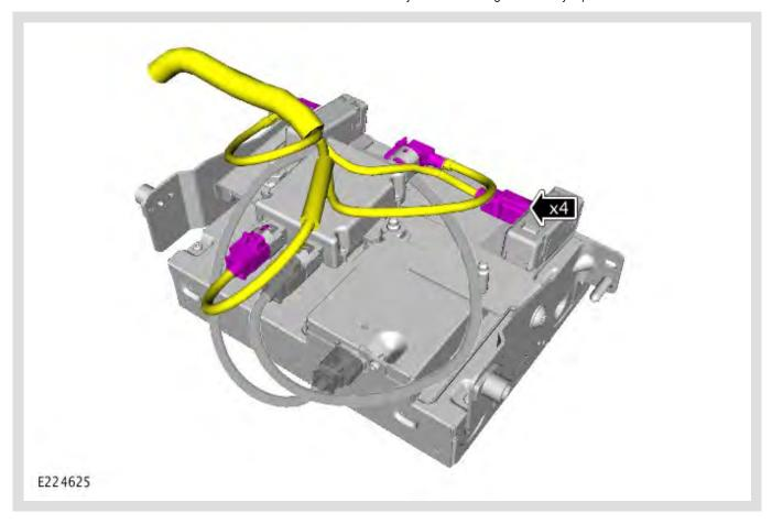
Install the electrical connectors to the USB 2.0 hub and WiFi/Bluetooth™ antennas as shown
