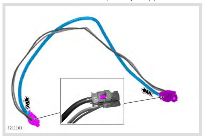
Release the electrical connectors from both ends of the original USB link lead.
