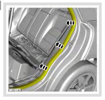
Reposition the rear left door aperture seal.
