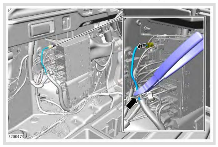
Remove the original IMC rear link lead cable connector from the Infotainment Master Controller (IMC).
