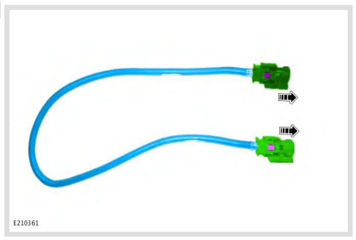
Release the electrical connectors from both ends of the new USB link lead.
