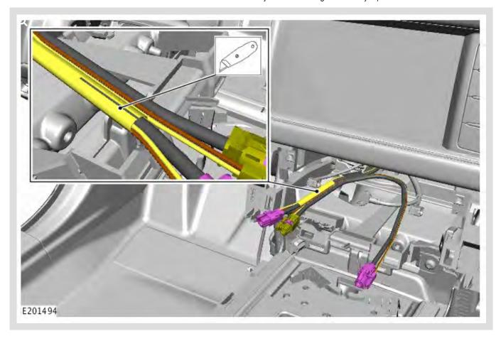
Use a suitable tool to remove some of the yellow tape on the IMC rear link lead for access.
