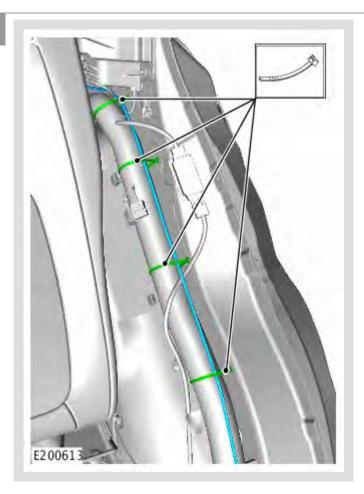
Route the new IMC rear link lead cable along the main harness above the wheel arch.
