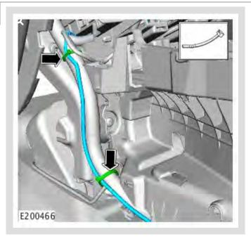
Route the new IMC rear link lead cable along the main harness towards the instrument panel.
