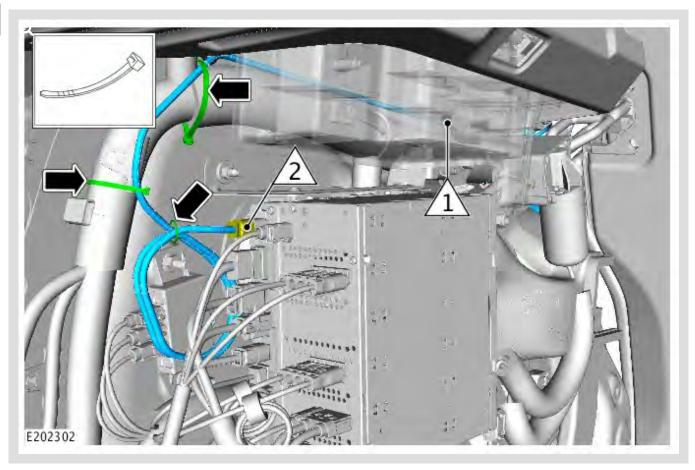
Install the same color connector on the new IMC rear link lead cable (2) to the Infotainment Master Controller (IMC).
