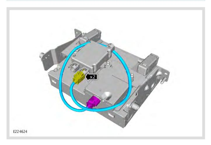
Install the electrical connectors to the digital disc player and USB 2.0 hub.
