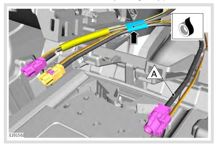
Install the new front link lead (A) and use suitable tape secure to the original wiring harness.
