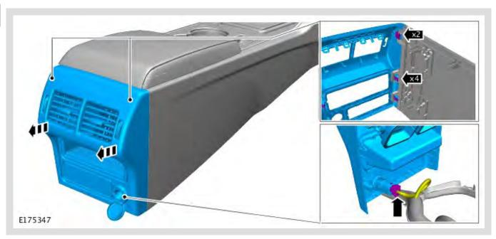
Remove the rear heater control panel.
