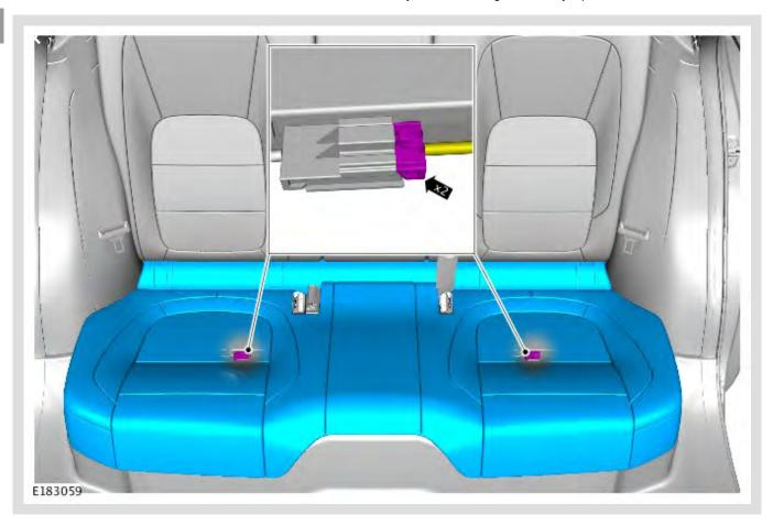
Disconnect the electrical connectors and remove the rear seat cushion.
