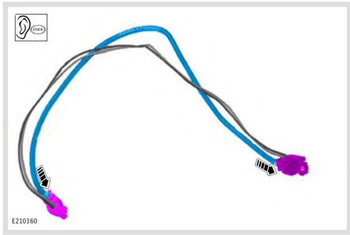
Install the replacement black coaxial USB link lead into the original electrical connectors.
