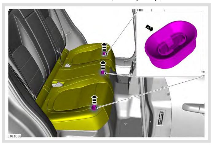
Release the rear seat cushion retaining clips.
