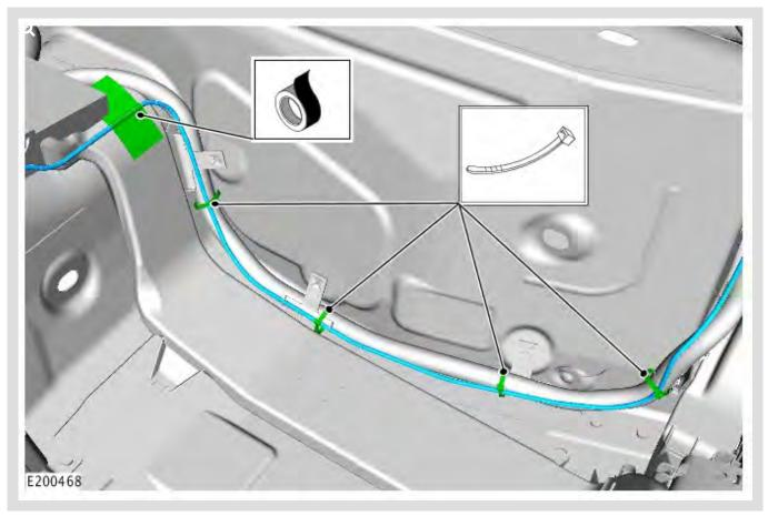
Route the new IMC rear link lead cable along the main harness in front of the rear seat base.
