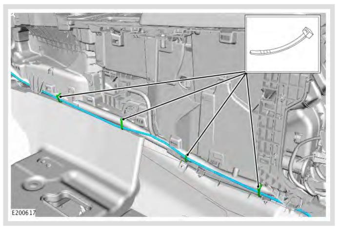
Route the new IMC rear link lead cable along the main harness below the floor console.
