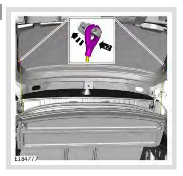
Disconnect the loadspace cover support straps.
