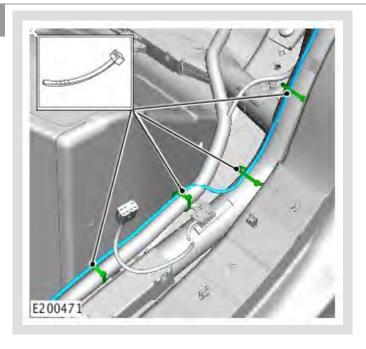
Route the new IMC rear link lead cable along the main harness below the rear door treadplate.
