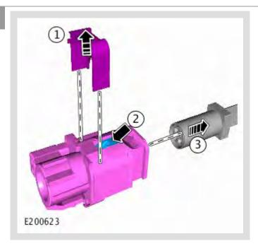
Using the sequence (1 - 2 - 3) in the illustration, remove the new rear IMC link lead cable from the new electrical connector.
