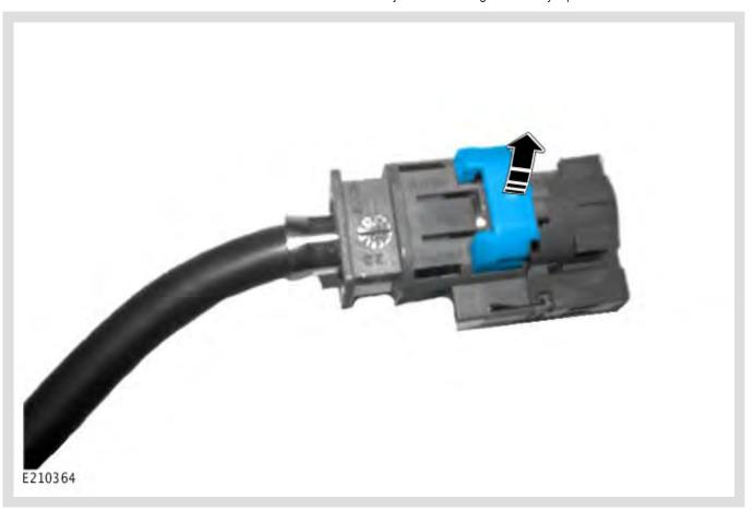
Use a suitable tool to remove the locking tab from the electrical connector at each end of the new USB link lead.
