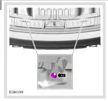
Loosen but do not remove the scuff plate lower nuts.
