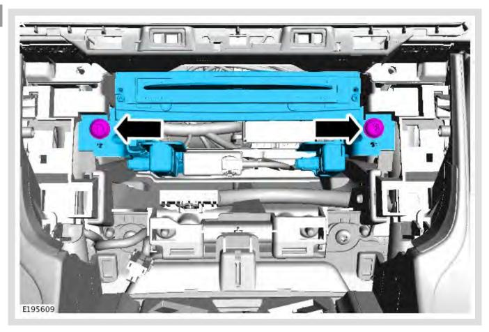
Remove the digital disc player, withdrawing the unit to view the wiring harness connections.
