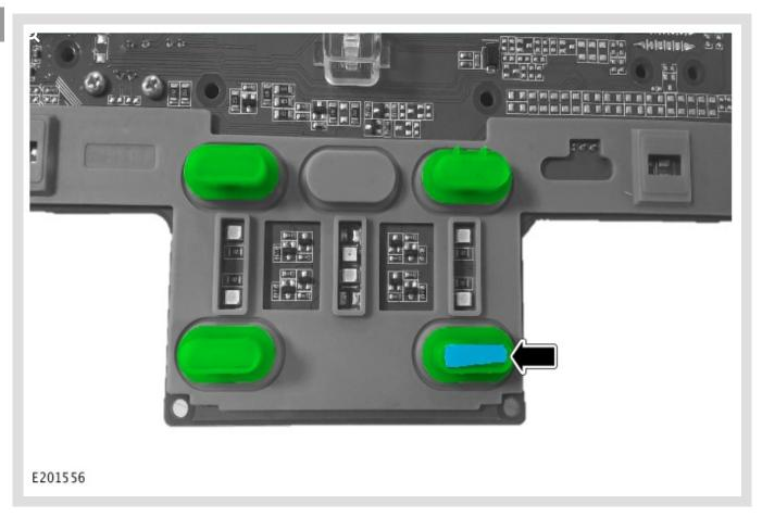
Install the 0.5 mm felt patch into this button as shown.
