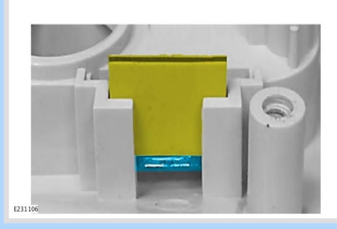
Make sure the conductive rubber strips make contact with the lower conducting element.
