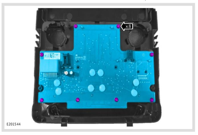
Remove the circuit board.
