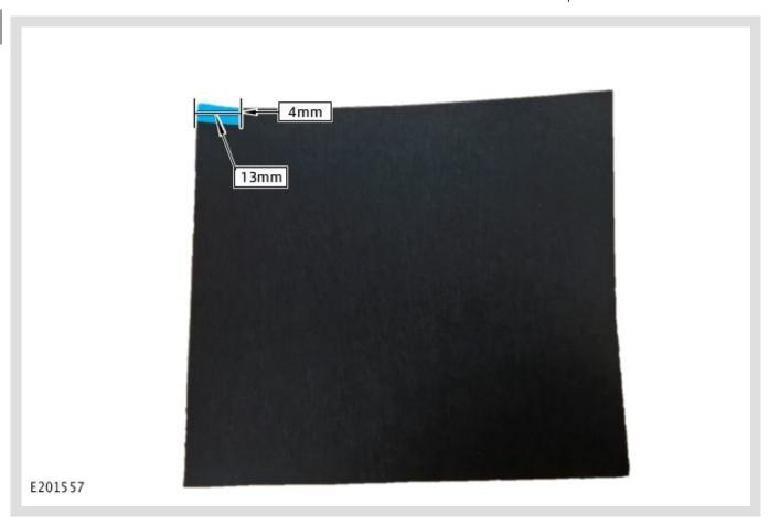
Cut a patch (13 mm  $\times$  4 mm) from the 0.5 mm felt sheet in the Jaguar Land Rover Squeaks & Rattles kit.
