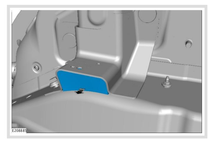
Remove the foam Noise, Vibration and Harshness (NVH) insulator.
