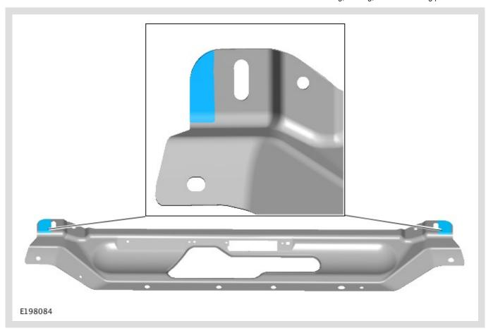
Cut 2 lengths of 1.6mm thick felt tape and apply to the cross brace in the locations as shown .
