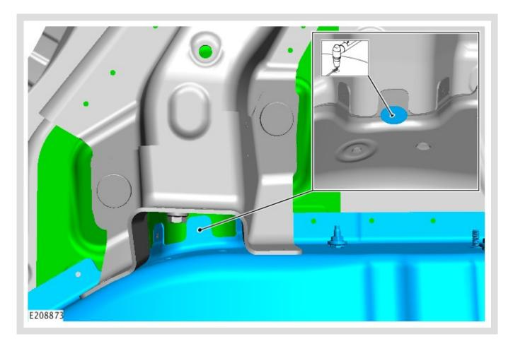
Use the appropriate welding equipment to apply a weld to the seam as shown.
