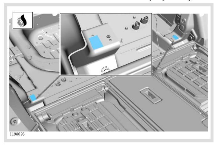
Cut 2 lengths of 1.6mm thick felt tape and apply to the panel as shown.
